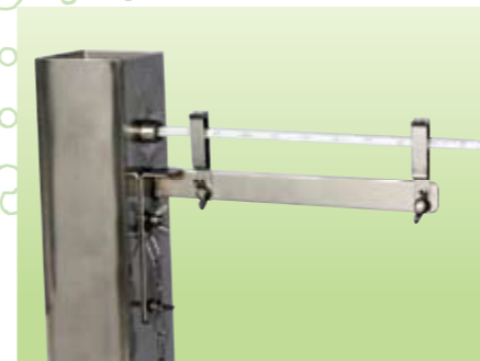
mercury thermometer and its holder
