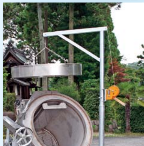
Equipped with a winch for shifting the heavy roof.
