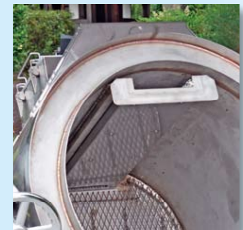
The shielding wall directs the heat waves to prevent burning the material, for the highest yield of charcoal.
