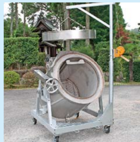
By turning the handle slightly, the kiln body can easily be inclined.
